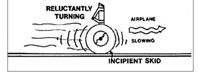
Whatever you do, don't lock the wheels. Braking effectiveness drops dramatically in a skid, and tires could be damaged.
