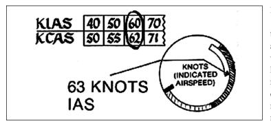
If you use CAS as Vso, however,  $1.3 \times 50 = 65$  knots CAS. Referring to the correction table, the IAS for an approach (at maximum landing weight in smooth air) would be 63 knots IAS, given an actual safety margin of 15 knots above the real, or calibrated, stall airspeed. The safety margin, however, will look like a margin of 23 knots on your airspeed indicator.
