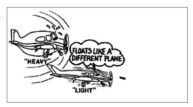
Remember, the 1.3 Vso formula is based on the actual weight of the aircraft, not the maximum landing weight. If you use your customary maximum weight 1.3 Vso number all the time, the aircraft will float as it dissipates the excess energy. Assuming that you will want to land at or close to the stall speed, runway distance will be eaten up during the process.
