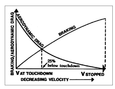
Apply brakes after all three wheels are on the runway and the airplane has slowed to at least 25 percent below touchdown speed. In fact, for most airplanes, aerodynamic drag is the single biggest factor in slowing the aircraft in the first quarter of its speed decay. Brakes become increasingly effective as airspeed and lift decrease.
